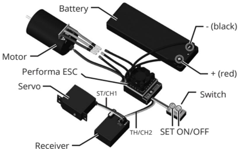
**Sensorless brushless motors:** When using a motor without sensors, if the motor spins in the wrong direction, simply reverse two of the motor wires.
